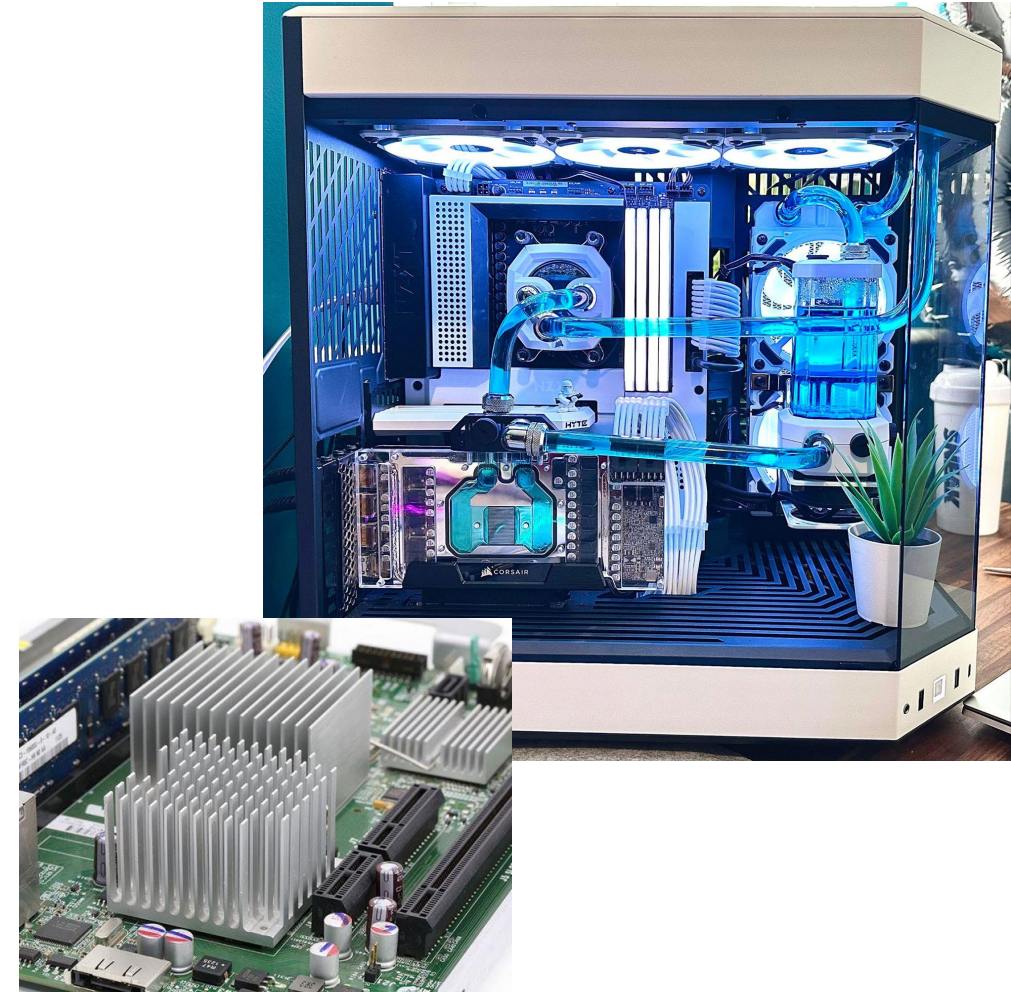
Cooling systems of all sizes include fans, heat sinks, and water loops, these also take energy to operate.
